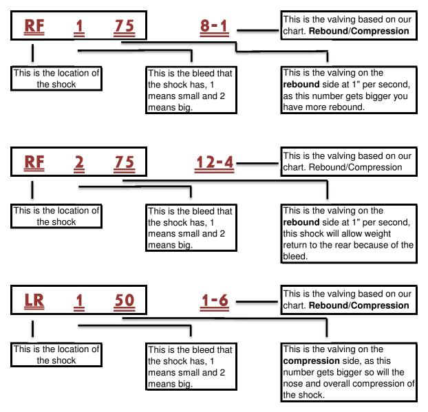
When we reduce the amount of bleed in a shock (1) the nose or low speed will increase in the shock, also the zero force increases too. As the zero force goes up, the cars ability to make front grip will decrease meaning you will want more bleed and more rebound. This is where the (2) bleed shock will out perform the other shock
